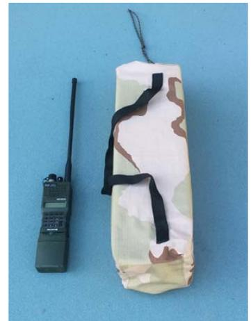
Fig. 1. LP MBWA ensemble for omnidirectional coverage in a camouflage bag beside an Army multiband radio AN/PRC-152.
